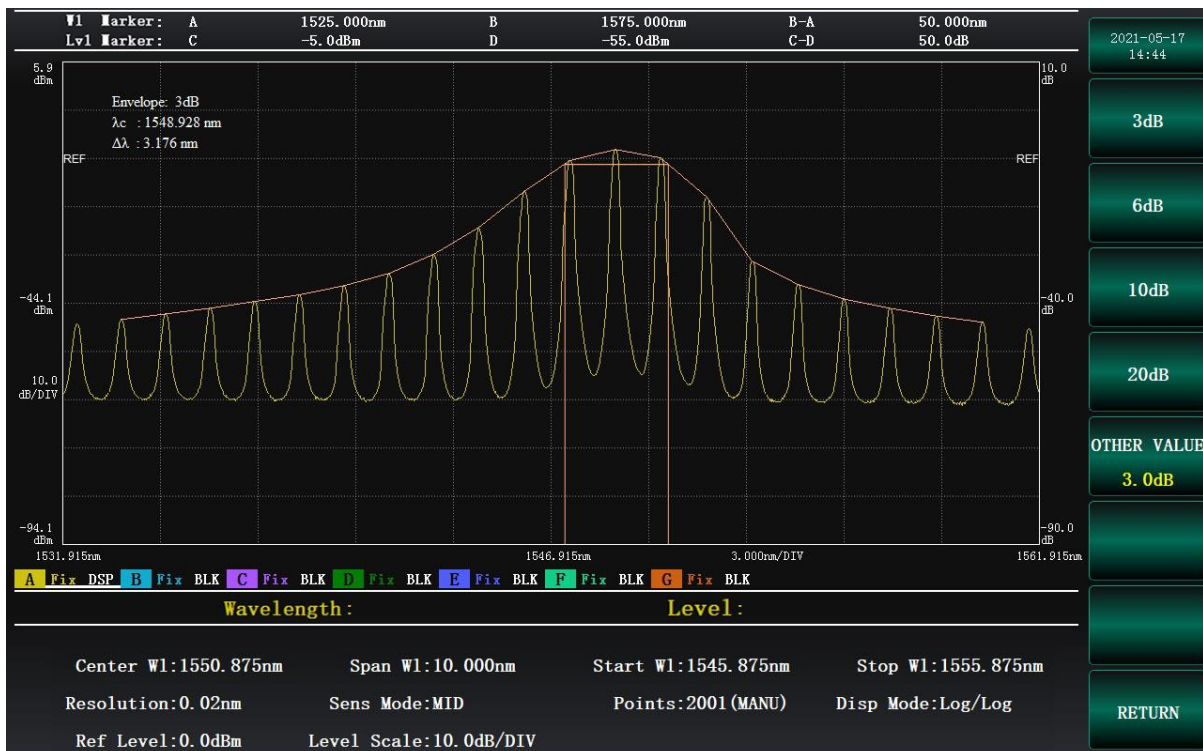
Center wavelength and bandwidth test based on envelope analysis
